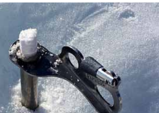
Figure 2. Taking an ice sample from the glacier. The samples were taken using ice-screws inserted 20 cm into the glacier surface.
